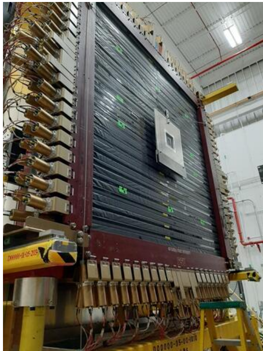
Figure 2.16: The TOF detector in Hall D mounted on its support frame. Source [38].
