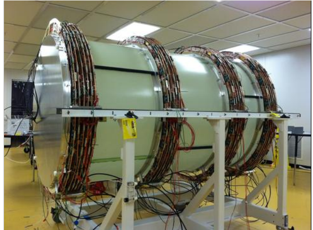
Figure 2.19: Left- Schematic representation of the FDC chamber showing the components. Right - The four mounted packages of FDC chamber. Source [13].
