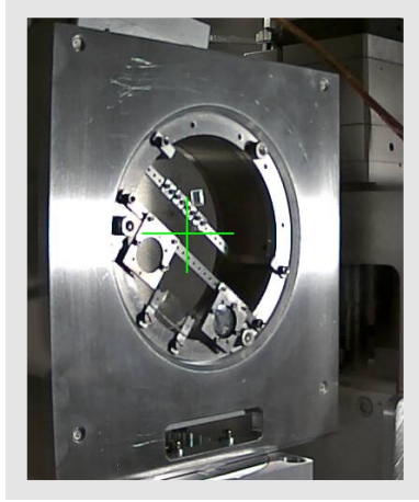
Figure 2.5: A picture of the goniometer. The diamond radiator is mounted in the centre. [41]
