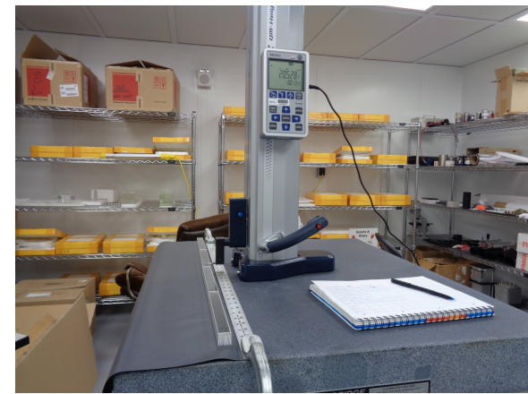
Mitutoyo tool ~ 7um accuracy on AA granite
