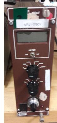
9. Turn on the DAQ system with the switch on the lower left of the power supply on the front.
