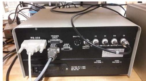
10. Turn on the controller for the horizontal translation stage motor. The switch for the controller is on the rear in the lower right corner.
