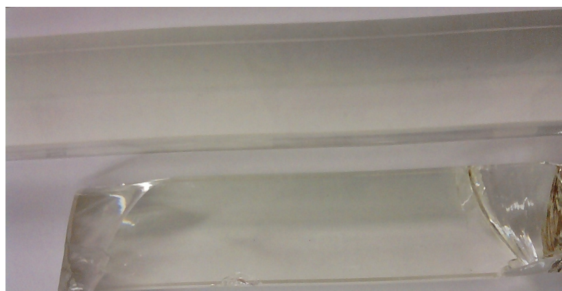
Figure 21: Photograph of F108, radiation hard glass. Top block is undamaged RHG and the bottom block is RHG dosed with about 700 kRad.
