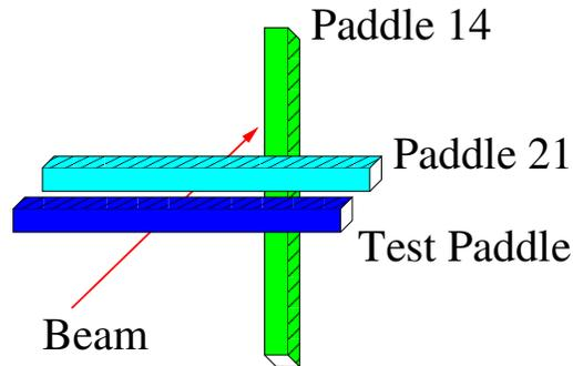
Figure 1: Schematic setup of the test paddle with respect to the horizontal and vertical TOF planes.
