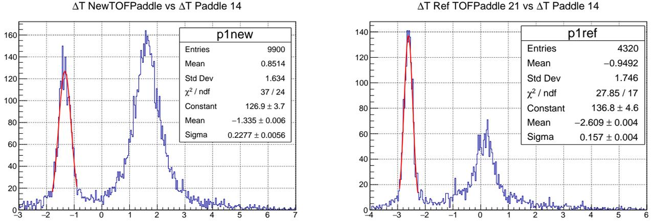
Figure 3: DT timing resolution for both the test paddle and paddle 21.
