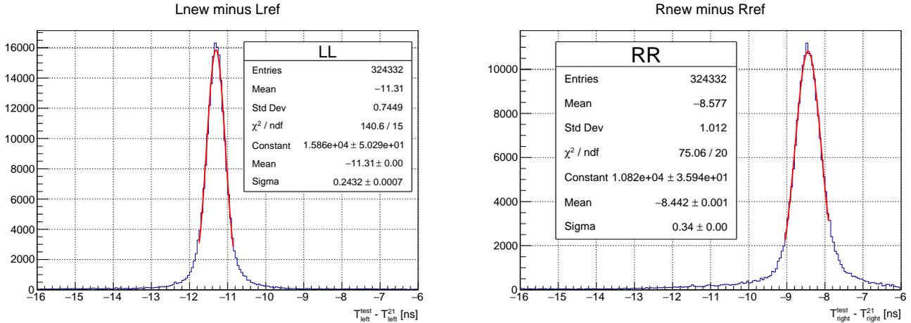
Figure 4: Time differences of the two left PMTs and the two right PMTs, respectively.
