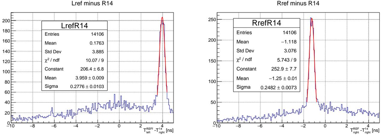
Figure 6: Time differences of the left and right PMT of the reference paddle 21 with respect to the right PMT of paddle 14.
