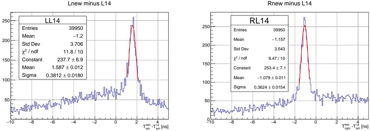
Figure 5: Time differences of the left and right PMT of the test paddle with respect to the left PMT of paddle 14.
