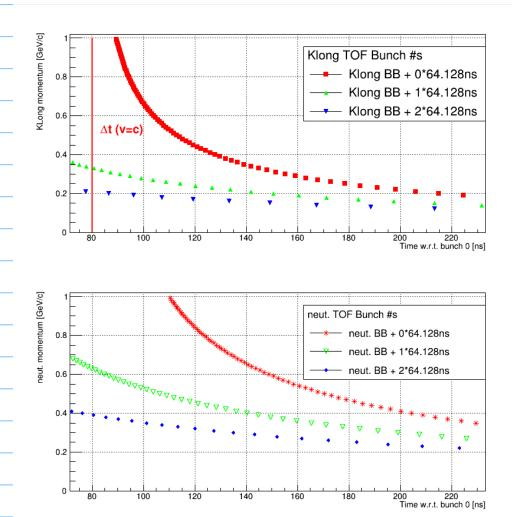
This shows that for a measured TOF of 120ns the expected Kaon momenta are 450MeV/c, 250MeV/c and 180MeV/c while the neutron momenta are 850MeV/c, 450MeV/c and 300MeV/c.
