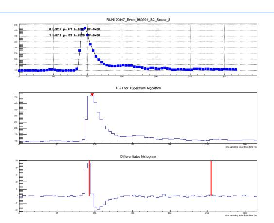
All the above wave forms are from run 120847, data taken with the nominal beam current on target. In the following we look at wave forms from run 121039 with a three times high beam current. Similar conclusions can be drawn here. However, it seems that the low readout threshold causes more wave forms with small signal amplitudes almost like noise.
