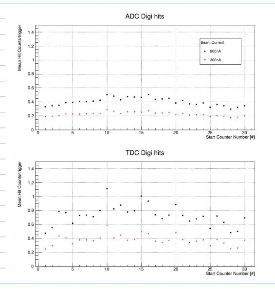
it is evident that the rates in the detector are higher for the 900nA beam which is expected. The threshold in the discriminator is set lower than in the flash ADC (w.r.t. base line) give by the fact that the rates are higher in the TDC than in the ADC. In some cases as high as 1 or more which means every trigger has a hit in that counter (10 and 15).
