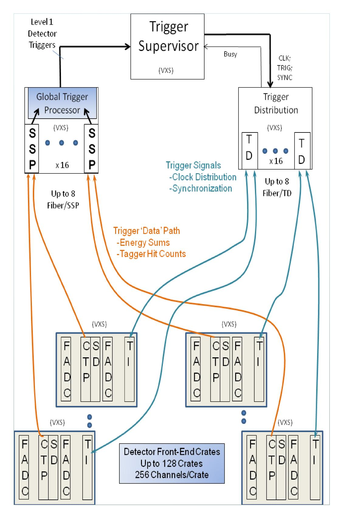
Two lanes @2.5Gbps from each FADC250 *payload* module are transmitted to the **CTP** *switch* slot using Xilinx's Aurora protocol on the VXS backplane. The energy sum transfer rate is 500MB/s from each FADC250 *payload* module to the **C**rate Trigger **P**rocessor *switch* module.
