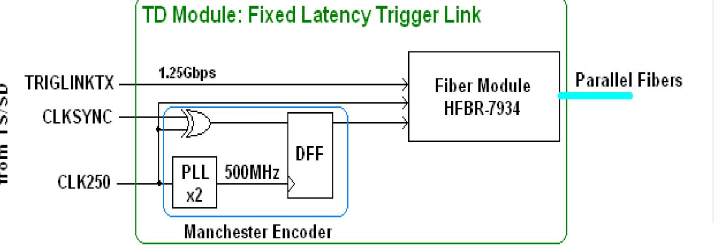
The fiber module is a POP4 compliant 4 channel Rx/Tx fiber module with 4 lanes @ 3.125Gbps per lane using 8b/10b encoding/decoding. This device is compact and can interface directly to Xilinx Virtex V Gigabit Transceivers. We have tested our system with fiber lengths of 50m and 150m to show the performance, and the longest fiber length that will be used in the experimental areas is <150m.
