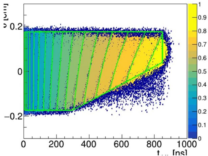
Run 50766 Predicted Drift Distance Vs.  $\delta$  Vs.  $t_{\text{drift}}$ , FOM 0.9+
