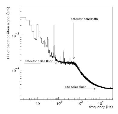
FFT coefficients (magnitude) of the x beam position signal taken while the photon beam is within 2.5 mm of the center of the collimator axis. Prominent peaks are seen in the spectrum at 30, 60, 120, 180, 198, and 360 Hz, corresponding to different modes of beam motion. The edge near to 600 Hz shows the bandwidth of the preamplifier at the gain setting used in this measurement.
