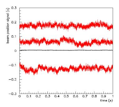
Photon beam centroid x position signals (red) formed from difference/sum of the two inner wedges, converted to cm. The traces were taken at different offsets of the beam from alignment on the central axis of the collimator. The reference trace (black) formed from measurements taken without beam present indicates the level of detector and electronics noise
