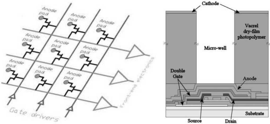
**Figure 2.** The pixelized micro-well detector concept. *Left:* Readout of a pixelized detector using a TFT array. The gate drivers are activated sequentially, allowing each column to be read out in turn by the charge-integrating front end electronics. *Right:* Cross section of a single integrated a-Si:H TFT/micro-well detector pixel. The drift electrode is not shown. The vertical scale is exaggerated.
