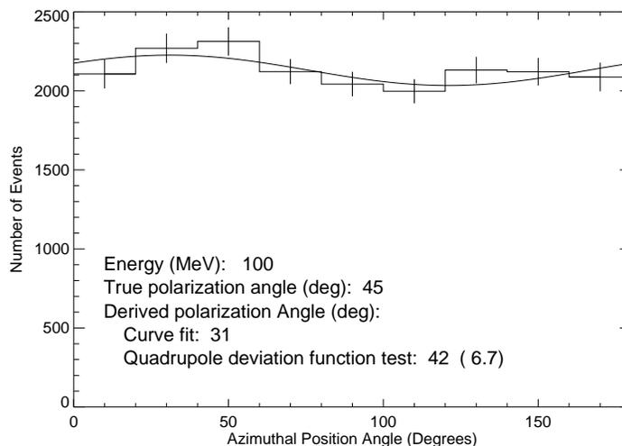
**Figure 6.** Azimuthal distribution obtained from Geant4 after applying detector response and event reconstruction routines. Only event within the 68% angular radius are included, given a total of  $\sim 1.9 \times 10^4$  events. The initial polarized distribution was divided by a normalized unpolarized distribution to remove systematics effects. The modulation factor is  $Q_{100} = 0.045$ .
