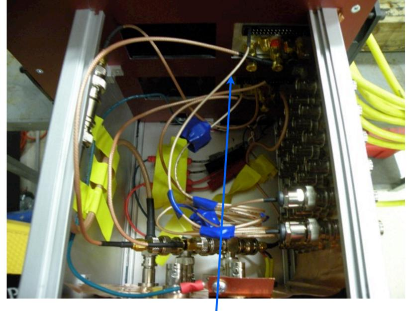
signal from preamp going to signal panel
