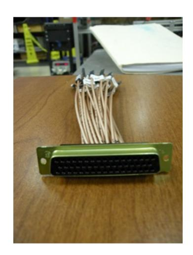
connects to output of detector signals
