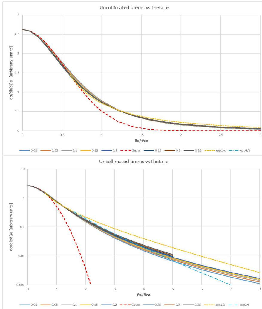
**Figure 1.** Solid curves: scaled angular distribution  $d\sigma/dk d\Omega_e$  versus  $\theta_e/\theta_{ce}$ . Dashed curves: Approximate fits to the angular distribution valid for the regions  $\theta_e/\theta_{ce} < 0.6$ , 0.6-1.6, and 1.6-10.
