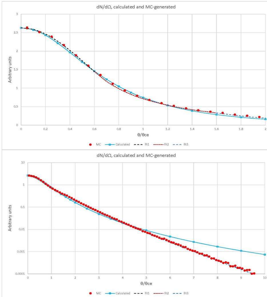
**Figure 2.** Solid curve: Calculated bremsstrahlung angular distribution  $d\sigma/dk d\Omega_c$  for  $E_c/E_0 = 0.2$  (other values very similar.) Dashed curves: Analytical functions of Section B in the 3 regions, 0-0.6, 0.6-1.6, 1.6-10. Points: Histogram of Monte-Carlo-generated distribution of  $dN/d\theta$  divided by central value of  $\theta$  for each bin.
