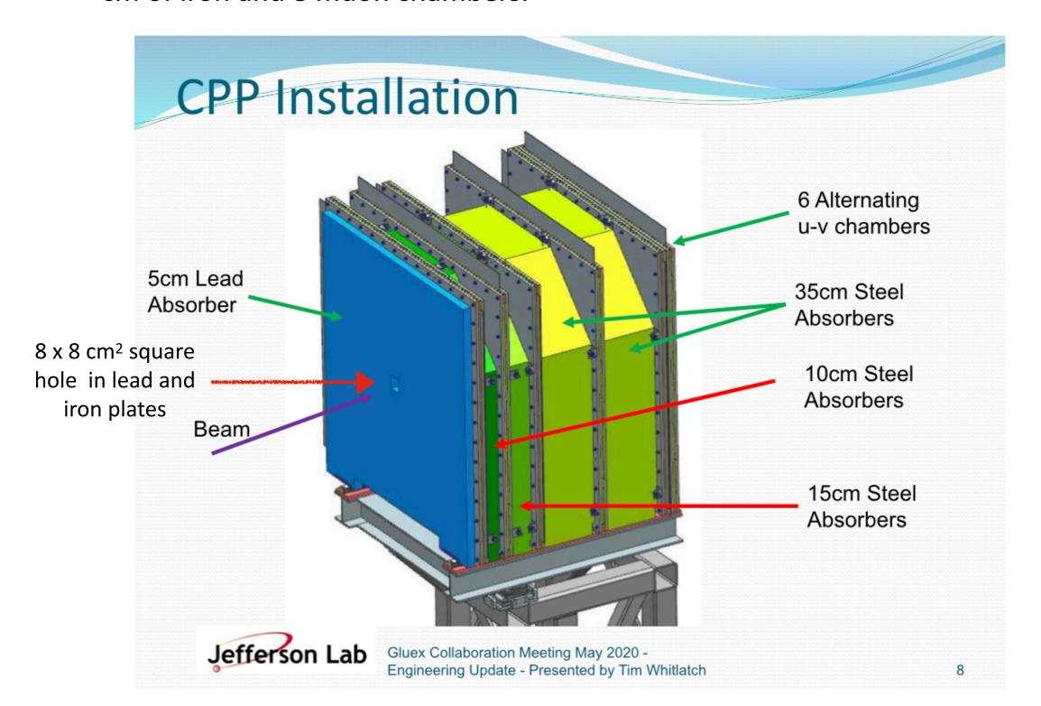
Design for detector and shielding installation in Hall D
