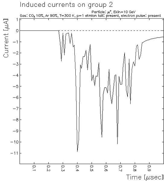
Fig 1.8 – Sense wire current at Full Scale, IP = 0.95 cm
