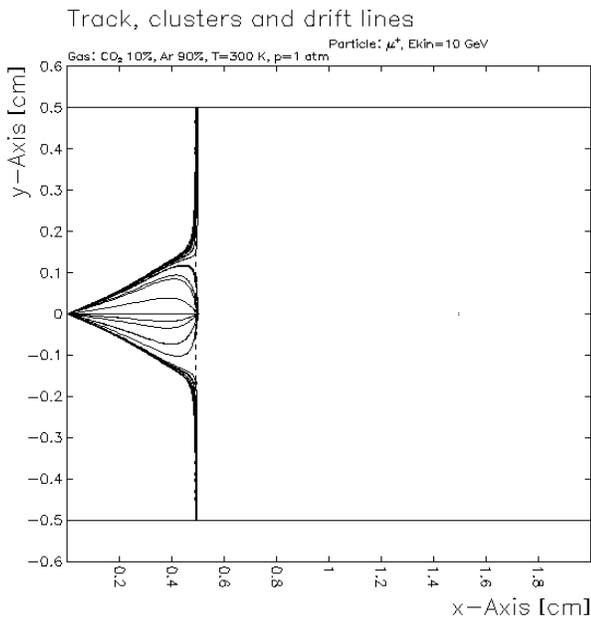
Fig 2.3 – Drift Tracks at Half Scale, IP = 0.25 cm
