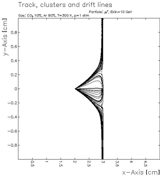
Fig 1.7 – Drift Tracks at Full Scale, IP = 0.95 cm
