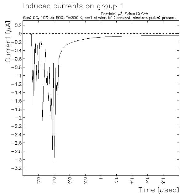
Fig 2.4 – Sense wire current at Half Scale, IP = 0.25 cm
