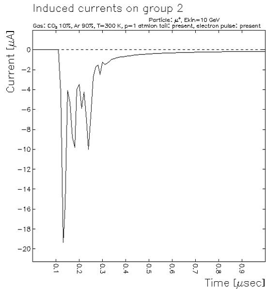
Fig 1.6 – Sense wire current at Full Scale, IP = 0.50 cm
