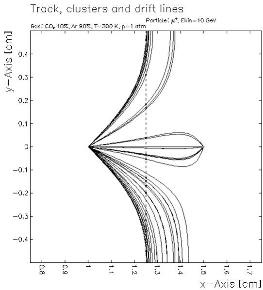
Fig 2.3 – Drift Tracks at Half Scale, IP = 0.25 cm
