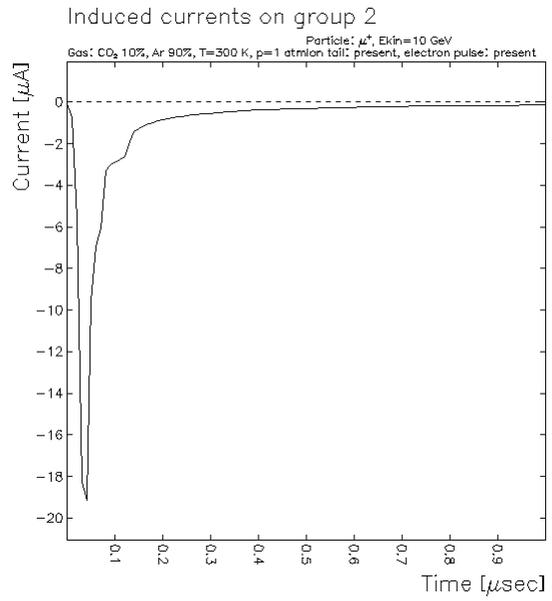
Fig 2.2 – Sense wire current at Half Scale, IP = 0 cm
