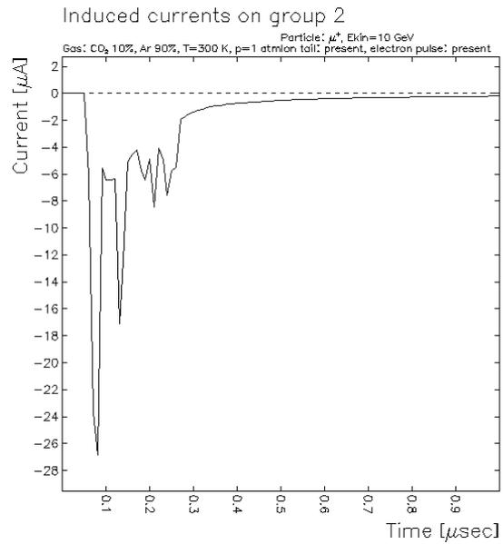
Fig 1.4 – Sense wire current at Full Scale, IP = 0.25 cm
