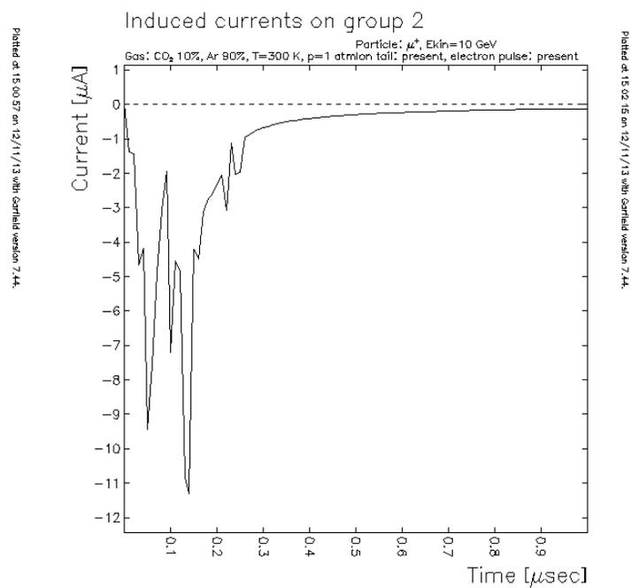
Fig 1.2 – Sense wire current at Full Scale, IP = 0 cm
