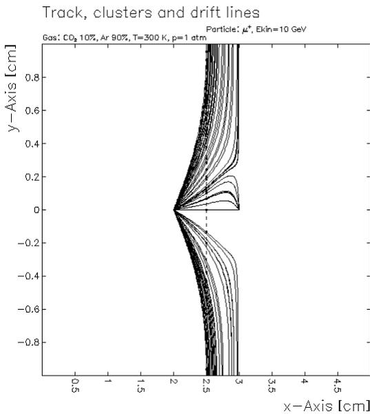
Fig 1.5 – Drift Tracks at Full Scale, IP = 0.50 cm
