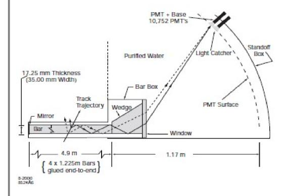
• Bars with rectangular cross section (radiators and as light pipes) for the portion of the light trapped in the radiator by total internal reflection
