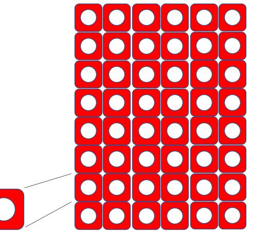
Conductor: 6 mm x 6 mm 4.5 mm hole Coil Construction: 3 double pancakes of 2 layers x 8 turns
