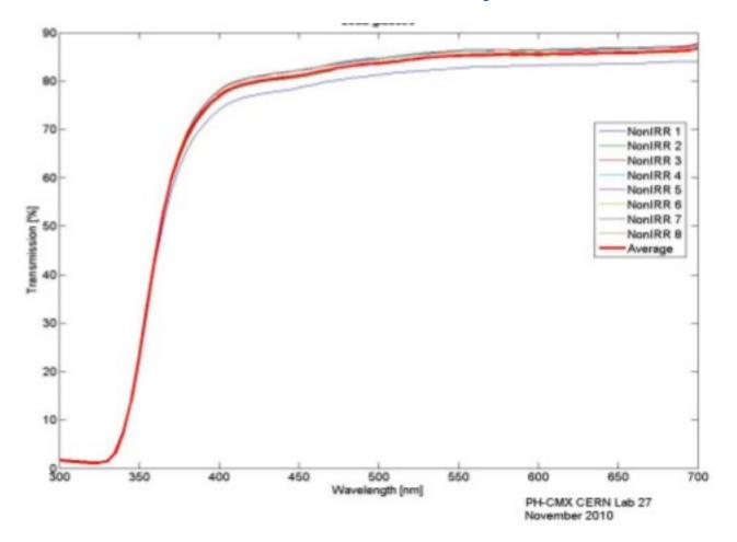
The < 100% transmission at long wavelengths is mostly due to light reflections at the two surfaces
