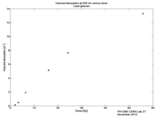
For a 30 cm SF5 block (X/X0 = 11.8) the light transmission T at  $\lambda$  = 400 nm after a dose of ~50 Gy is given by
