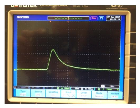
A minimum ionizing electron passing perpendicular to the wire plane deposits on average 5.0 keV of energy from atomic collisions. Approximately 192 electron ion pairs are produced along a 2 cm track.
