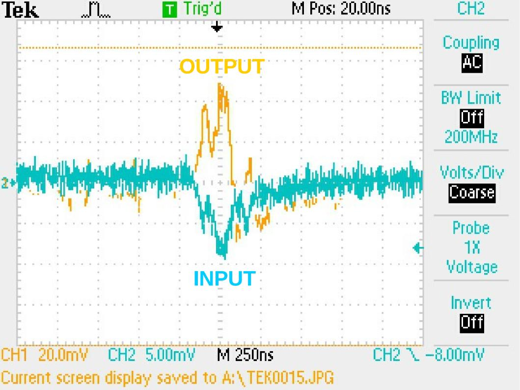
(Sine wave with frequency of 5.0 MHz and and amplitude of 3.5 mV through a blocking capacitor and then a 100 ohm resistor, expected current into amplifier ~35 uA)
