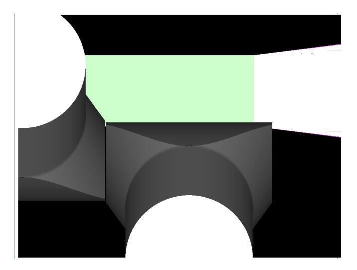
Another issue that I am noticing is that with the fishtailed light guides we may need to increase the space between the TOF and FCAL movable platform in regards to the mounting because of this also. It appears that the lightguides/shields in the vertical plane clip the corners now that they are angled verses straight. We may need to put a little more space in between them if possible.
