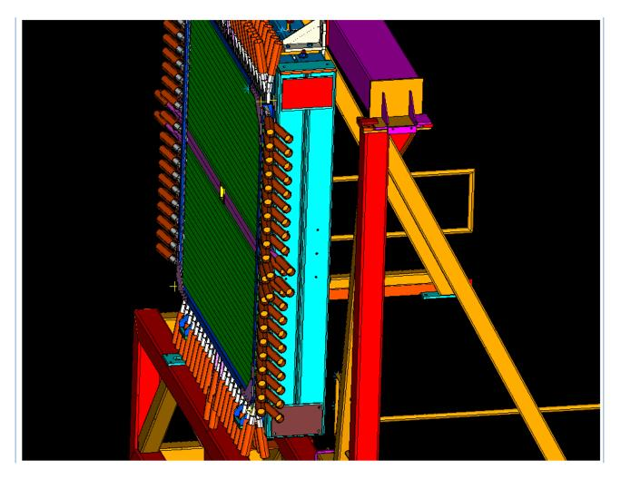
And last, the split lightguides stick out of course a lot further than the others. This may or may not be a problem in the bottom section as far as room for the wires etc, to come out. This is true only at the bottom of the TOF.
