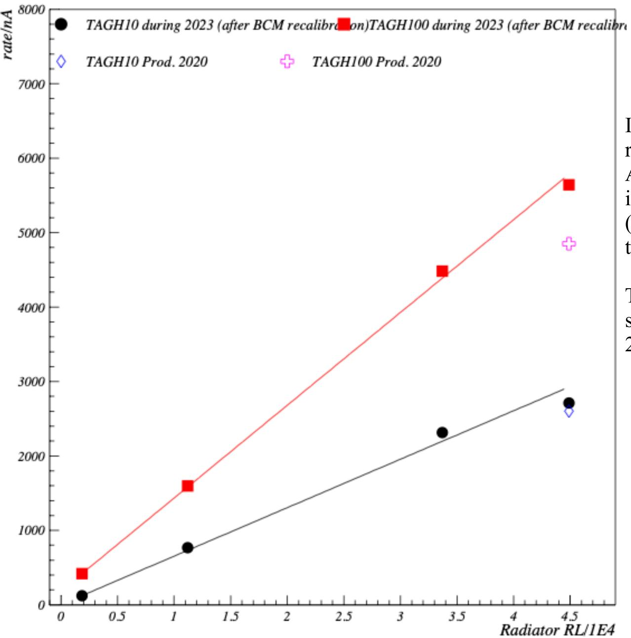
Initially, it was thought the  $\sim 30\%$  change in rate could be due to a radiator problem. Therefore, we checked the linearity of the yield with Al. radiator thickness, see figure. It appears linear as expected, making it very unlikely that there is a problem with the radiator, since all (goniometer+amorphous radiator ladder) would have to be affected in the same way.
