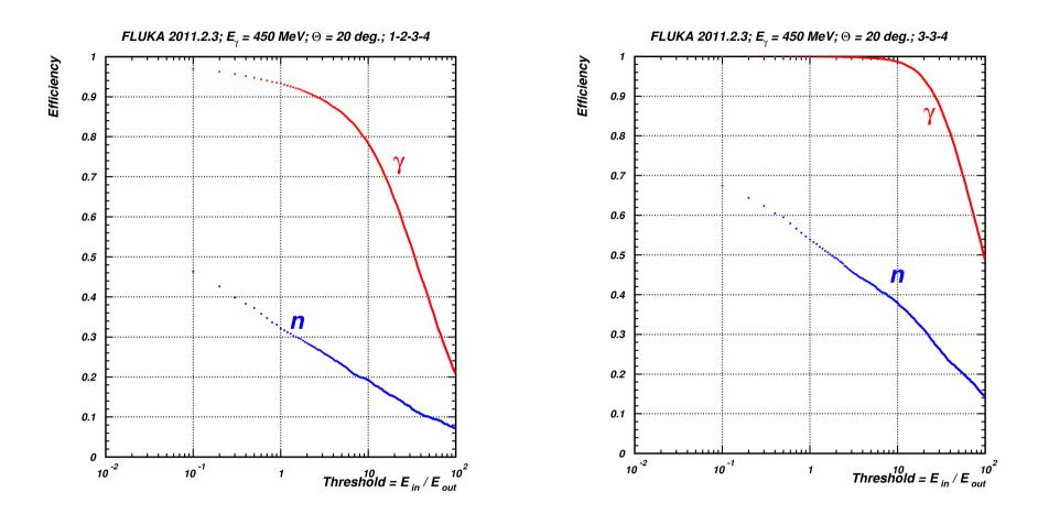
Suppression of neutrons by factor of about 2.5 is achievable without reducing the photon efficiency
