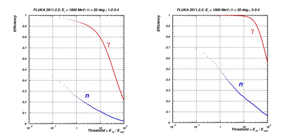
Suppression of neutrons by factor of about 4 is achievable without reducing the photon efficiency
