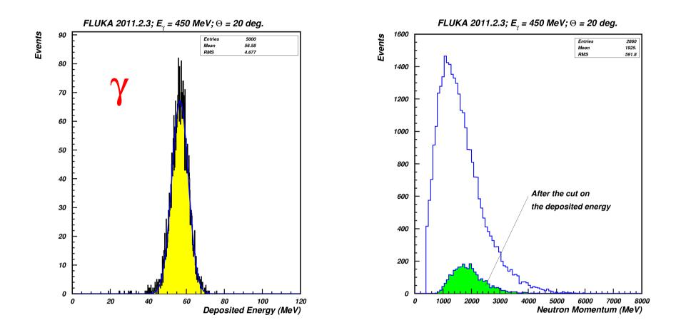
NOTE: Kinetic energy of selected neutrons (of about 1200 MeV) is significantly larger than the energy of correspondent photons.
