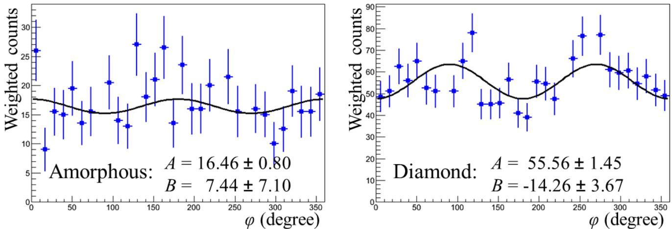
FIG. 7: Azimuthal distribution. Left panel: Azimuthal distribution for amorphous radiator (run 3180). Right panel: Azimuthal distribution for diamond radiator (run 3185). Each of the distributions were fit to the function  $A[1 + B\cos(2\phi)]$ , with  $A$  and  $B$  being parameters of the fit. The weighting of the histograms is described in the text.
