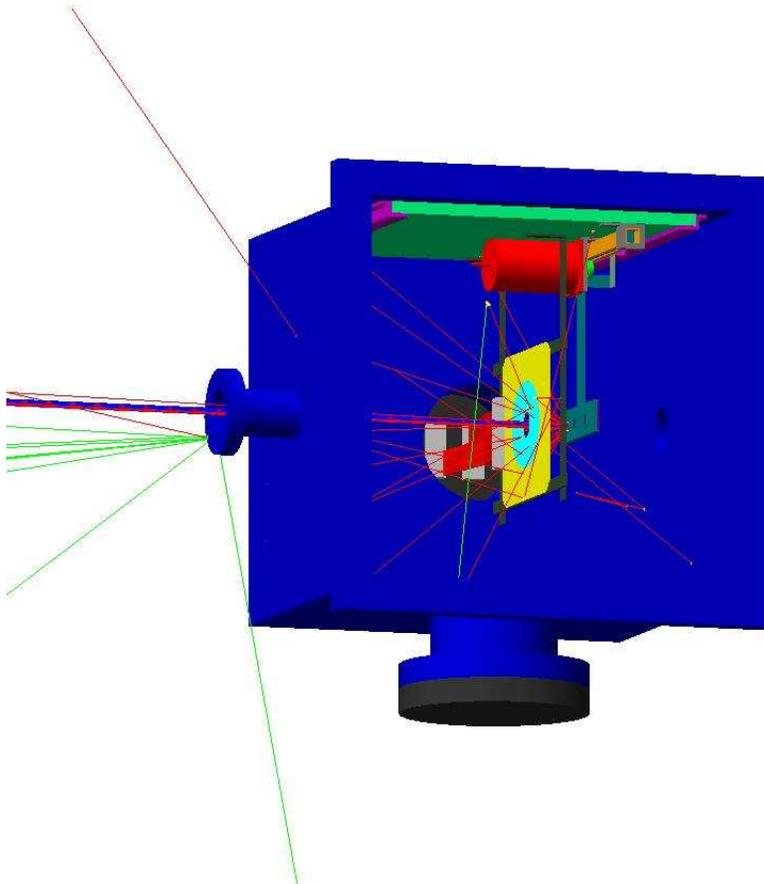
FIG. 3: Simulation of the triplet polarimeter with 100 thrown events.
