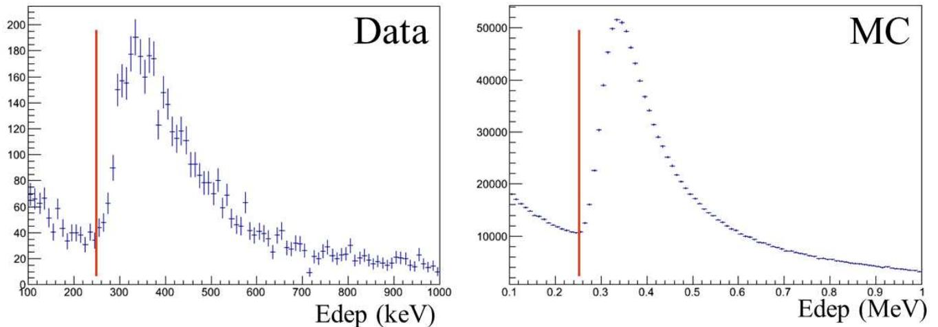
FIG. 6: Energy deposition in the polarimeter. Left panel: Energy deposition for real data (run 3185) where timed hits were weighted as unity and out-of-time hits were weighted by -0.5. Right panel: Energy deposition for Monte Carlo data. The red lines at 250 keV represents the energy cut made in the analysis.
