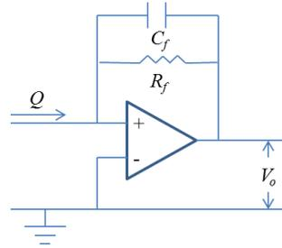
FIG. 2: Circuit diagram of a generic charge-sensitive preamplifier.
