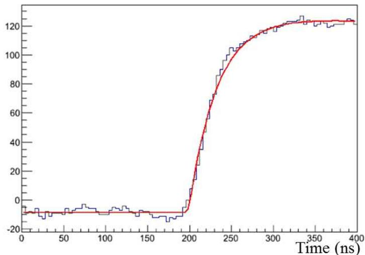
FIG. 4: Example fit to fADC signal versus time (ns) using the function described in the text.
