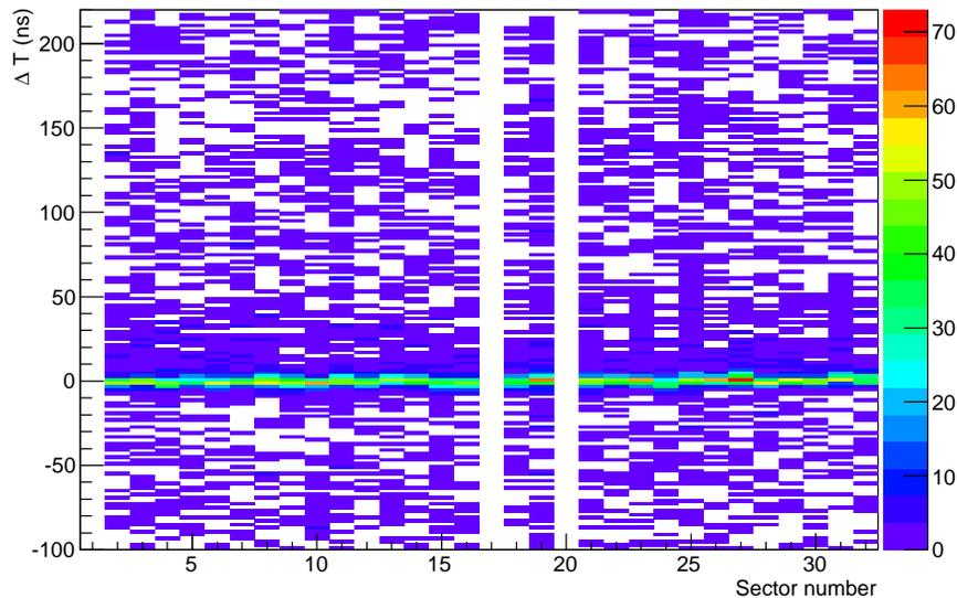
FIG. 5: Time difference between pair spectrometer and triplet polarimeter ( $\Delta T$ ) versus sector number of polarimeter.
