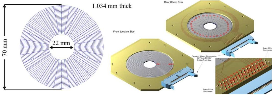
FIG. 1: The S3 double sided silicon strip detector.
