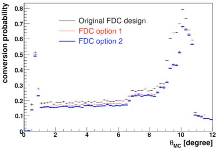
FCAL reconstruction efficiency; photon conversion probability as a function of angle.
