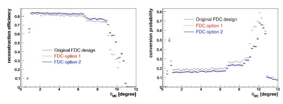
FCAL reconstruction efficiency; photon conversion probability as a function of angle.
