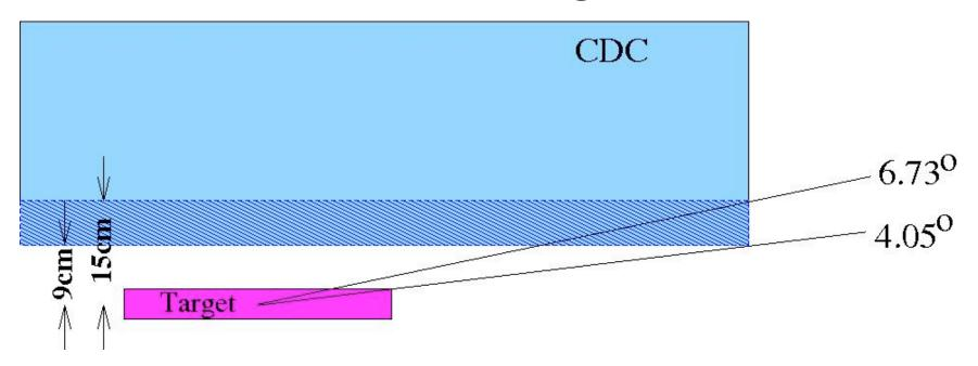
The bug was that the inner radius of the CDC was set at 9 cm instead of 15 cm. This placed additional material in the detector for tracks between 4.05 and 6.73 degrees.
