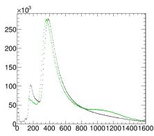
• Black is data and green is mc. Energy depositon (keV) on x-axis, counts on y-axis. Left is 10keV and right is 20keV smearing.
