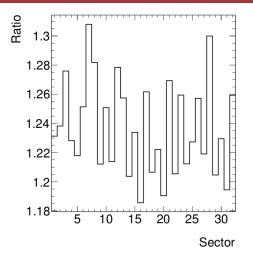
Took ratio between most probable value of landau fit to a sector's TPOL energy deposition to that of the max value in MC. Working on fitting MC, but enhacement beyond main triplet peak.
