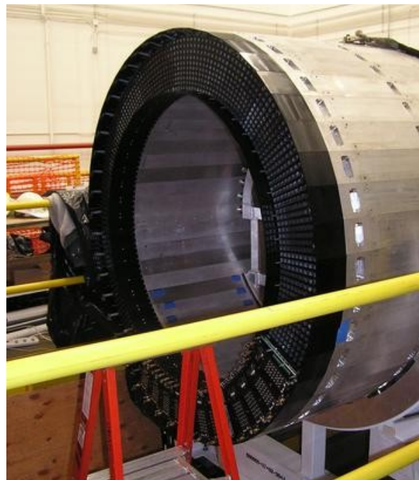
Barrel calorimeter 11^\circ < \theta < 125^\circ
