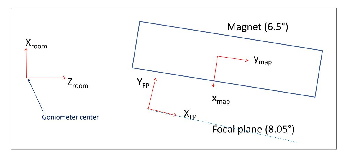
Since raytracing is done in map coordinates, I define the origin of the Focal Plane coordinate system to be fixed relative to the center of the magnet. Some facts about the new survey:
