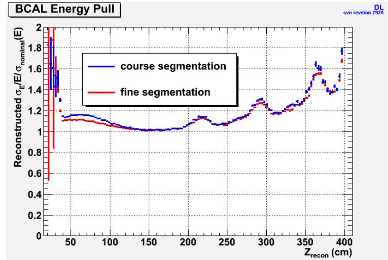
Dividing out each bin by the nominal energy resolution gives pulls indicating (in part) how well the simulated data follows that resolution function
