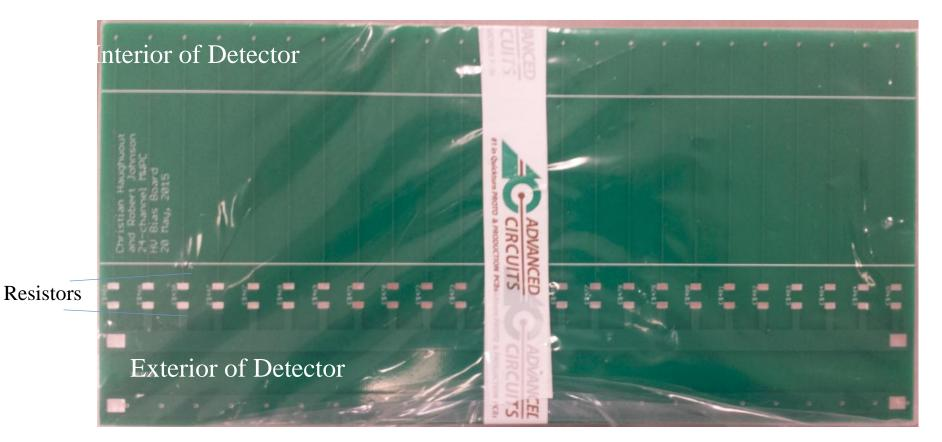
• Determine if there is enough clearance between resistor and aluminum plate to put resistors inside detector
