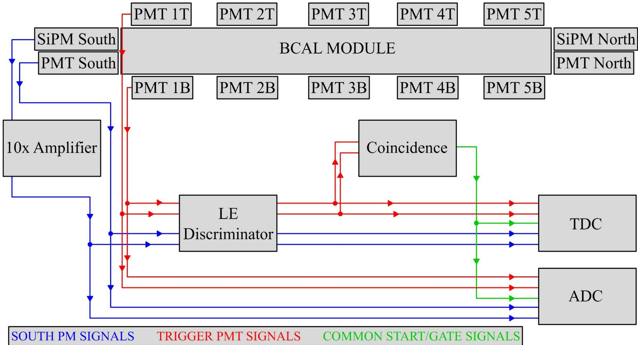
Shown for one trigger pair and the south photomultipliers. The other four trigger pairs and the north photomultipliers have identical setups
