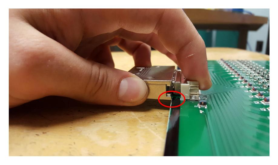
The issue that the breakaway rails being present on the board causes is that the connector cannot attach to the board as the lower portion of the cable hits the board material before a connection is made
