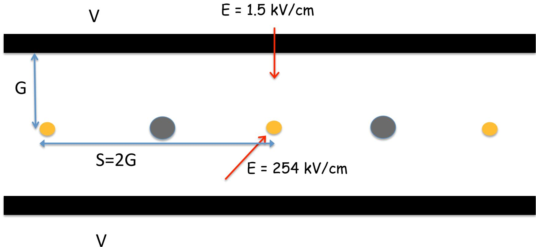
$E = 254 \text{ kV/cm}$  corresponds to a gas gain of  $10^5$
