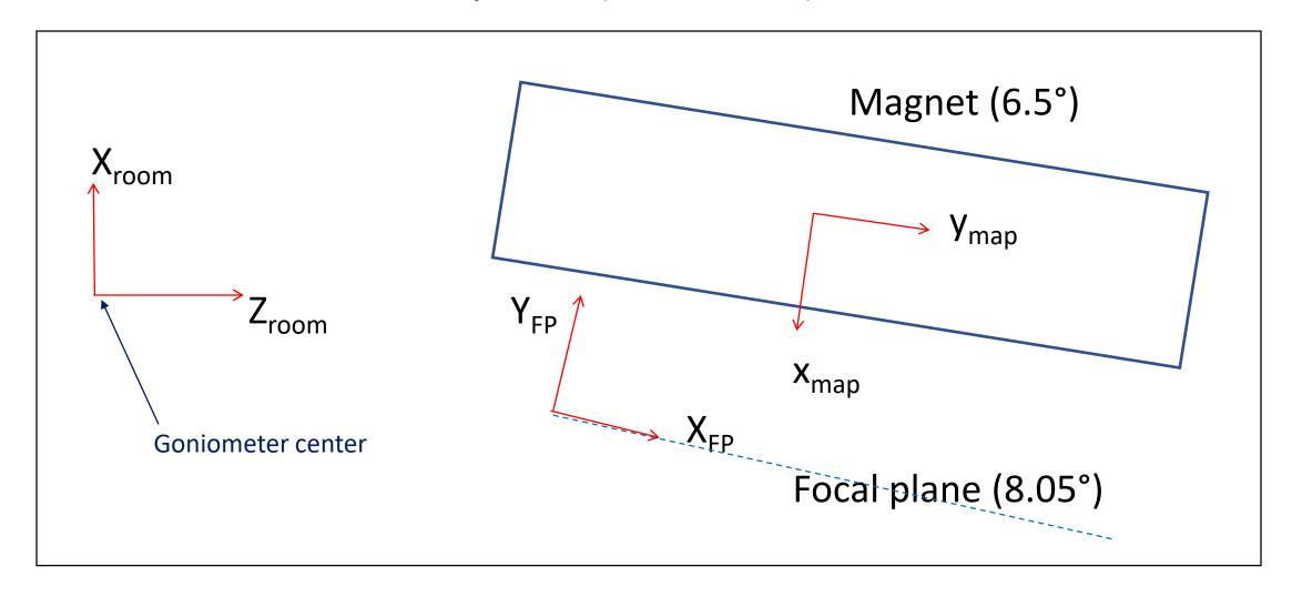
Since raytracing is done in map coordinates, I define the origin of the Focal Plane coordinate system to be fixed relative to the center of the magnet. Some facts about the new survey:
