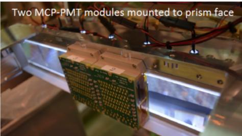
Removable optical coupling is made using a soft cast silicone cookie with a drop of optical oil to make a "bubble free" contact
