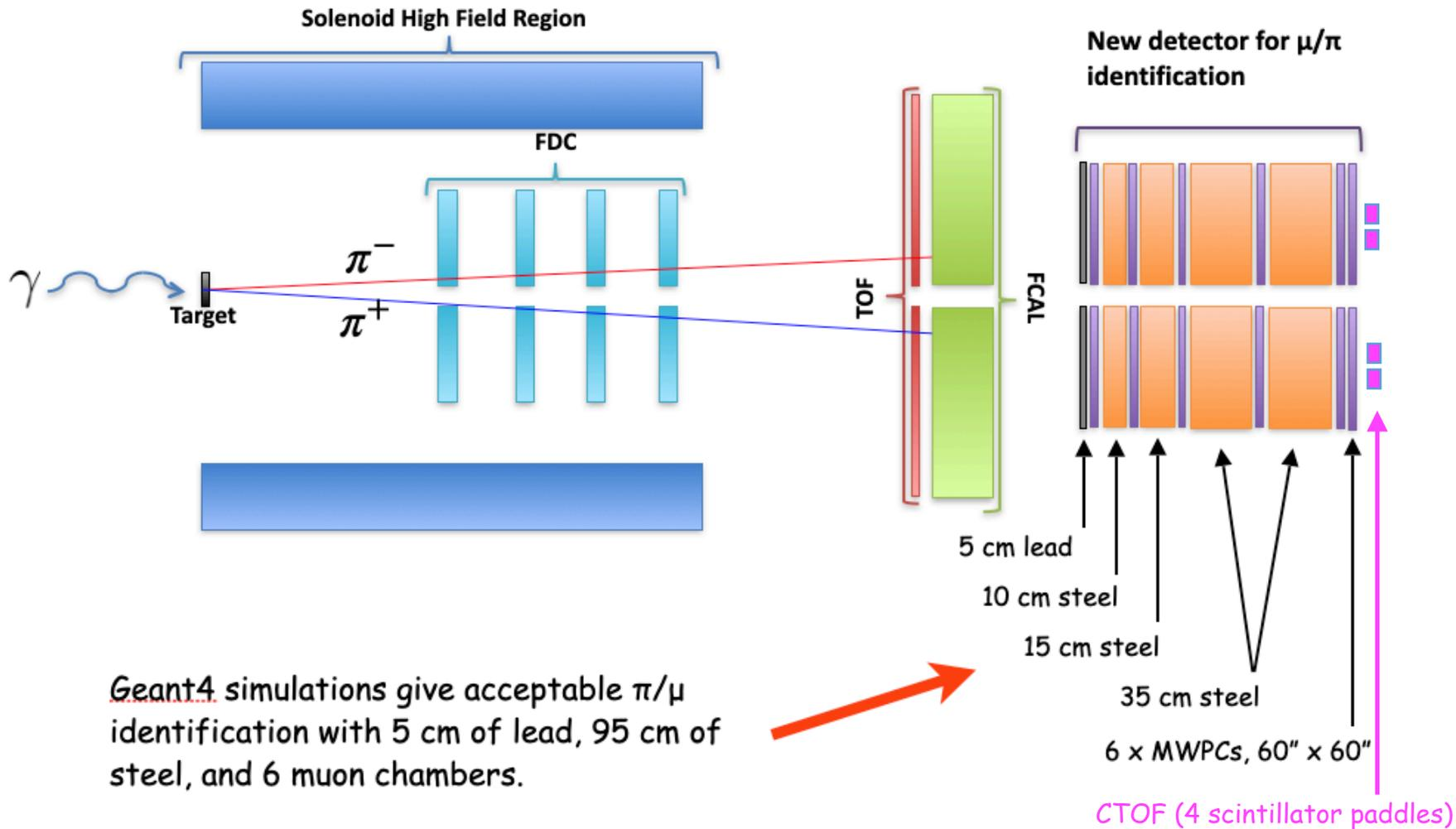
Geant4 simulations give acceptable  $\pi/\mu$  identification with 5 cm of lead, 95 cm of steel, and 6 muon chambers.
