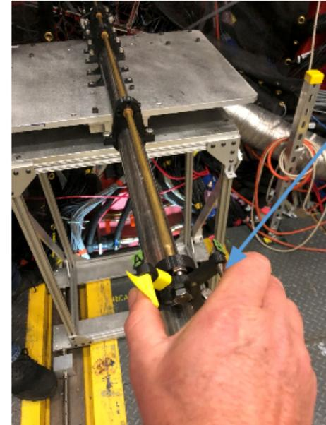
Grab threaded studs to rotate clockwise 90° to put lead in beam, rotate ccw 90° to put blank frame in beam
