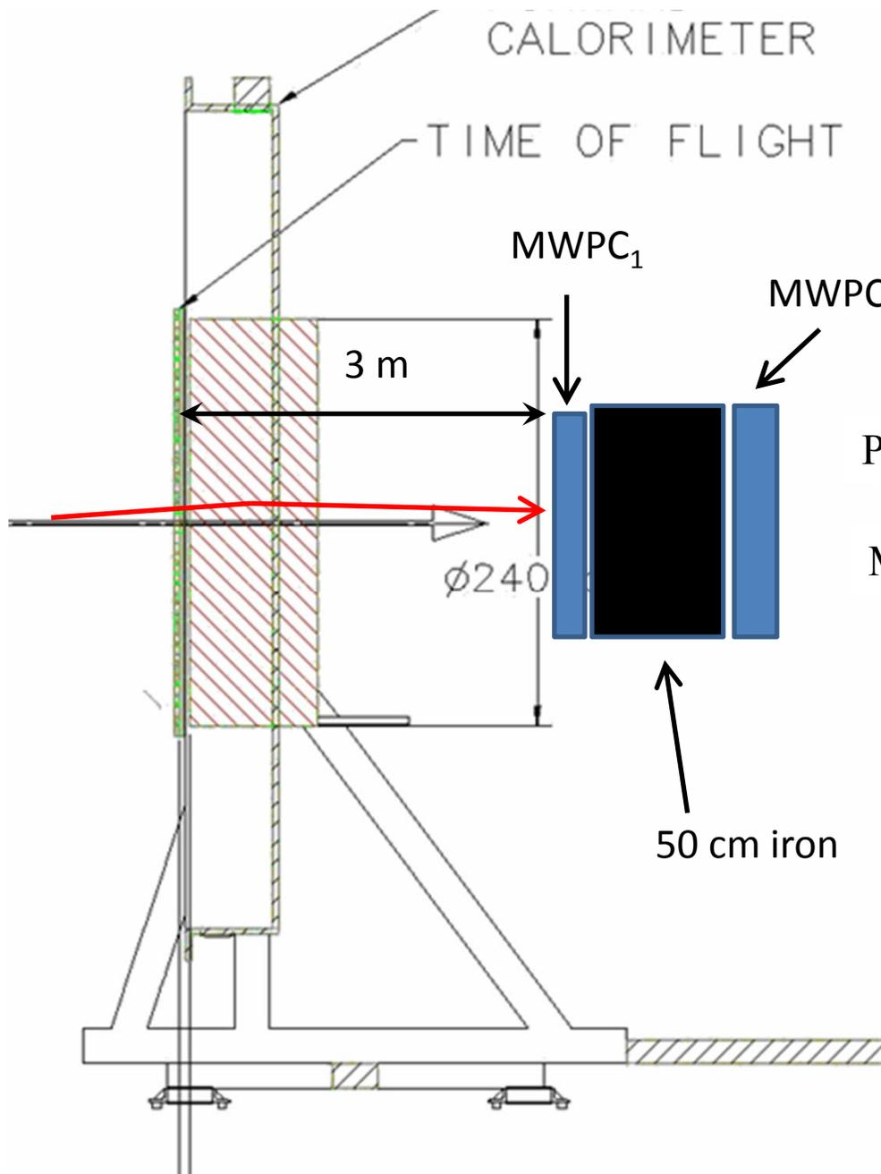
$$\text{Pion signal} = TOF \cdot (FCAL + MWPC_1) \cdot \overline{MWPC_2}$$
