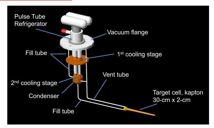
Liquid hydrogen (or deuterium) is condensed in the target cell, condenser, and fill & vent tubes. The liquid is subcooled 1-2 K below the SVP curve to suppress boiling.
