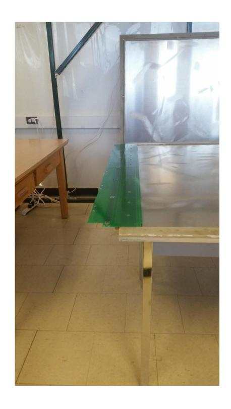
The sense boards have been epoxied to the bottom plate
