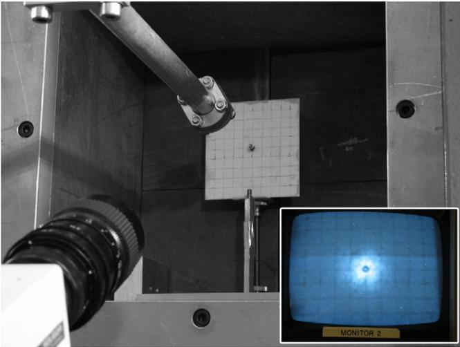
**Fig. 3.** Experimental set-up for SiPM irradiation. Electrons (14 MeV) left the evacuated beam-pipe through a 0.3 mm aluminum window. Multiple Coulomb scattering of the beam generated a wide spot on the fluorescent screen. The beam position could be accurately steered so that the SiPM was at the centre of the spot as can be seen in the on-line monitor picture (inset lower-right). The small SiPM active area was considered as uniformly irradiated.
