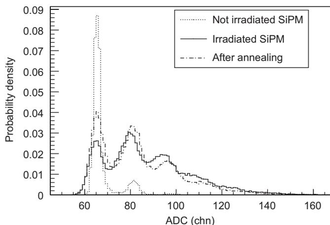
**Fig. 10.** Annealing at 80 °C of the SiPM exposed to the radiation field in the experimental hall resulted in a partial recovery. The ADC spectra for a randomly generated integration window of the green sensitivity SiPM are shown before and after irradiation. The same histogram is shown after the heat treatment.
