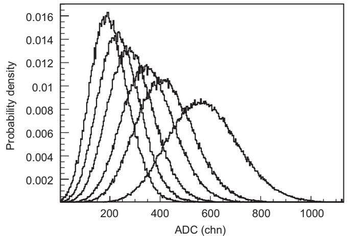
**Fig. 7.** ADC spectra for fixed laser intensity after irradiation with 30.8, 77.0, 123, 185, 262 and  $385 \times 10^8$  electrons. A progressive reduction of the photon detection efficiency or of the SiPM gain is suggested as an explanation for the observation of lower integrated charge with increased irradiation dose.
