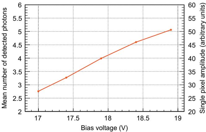
**Fig. 4.** Photon detection efficiency and gain as a function of the bias voltage for the green sensitive Photonique SiPM.
