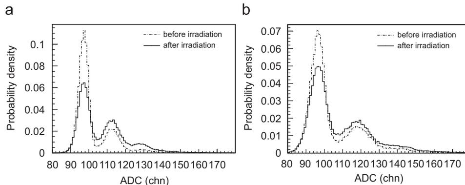
**Fig. 9.** Noise spectra of two blue sensitive Photonique SSPM-0611B1MM devices before and after irradiation in a mixed radiation field close to the beam-line. (a) SiPM without radiation shield. (b) SiPM shielded by 3 cm of BPE and 2 mm of lead. A reduced damage was observed for the shielded SiPM.
