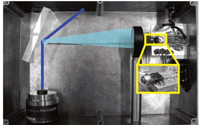
**Fig. 2.** Experimental set-up for SiPM characterization: a fast pulsed UV laser (100 ps FWHM) excited a plastic scintillator. Reflected UV light was absorbed in a black screen. The blue scintillation light was attenuated by a neutral density filter so that only few photons arrived to the SiPM (inset right).
